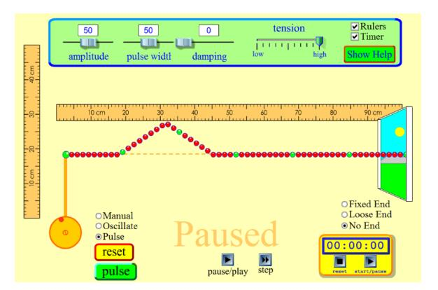
With the **tension** setting at **high**, press the **pulse** button and the quickly hit the **pause/play** button and the **step** button to obtain distance and time data for the motion of the pulse.
