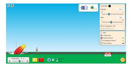
Use the settings Cannonball Diameter, Cannonball Mass, and Air Resistance to launch the cannonball. Drag the crosshairs marked with time and range to the spot where the pumpkin landed. Then drag the crosshairs to the top of the parabola to find max height. Fill in the table below with the values.
